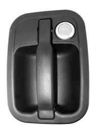
This flush mount pull handle was specifically designed for compartment and entrance doors for off-highway vehicles. It offers ergonomic function and styling, is adaptable for power door lock actuation and has a "locked-rigid" handle when locked. The design provides for ease of operation by keying alike with other Tri*Mark* products with the KeyOne™ Plus lock.
